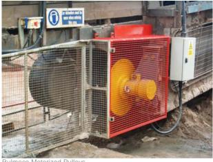
Rulmeca Motorized Pullevs
